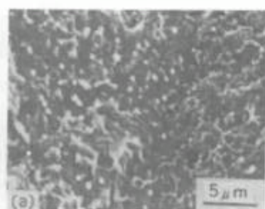
Fig.4 SEM of fractured surface of composite prepared by in-situ blend.
